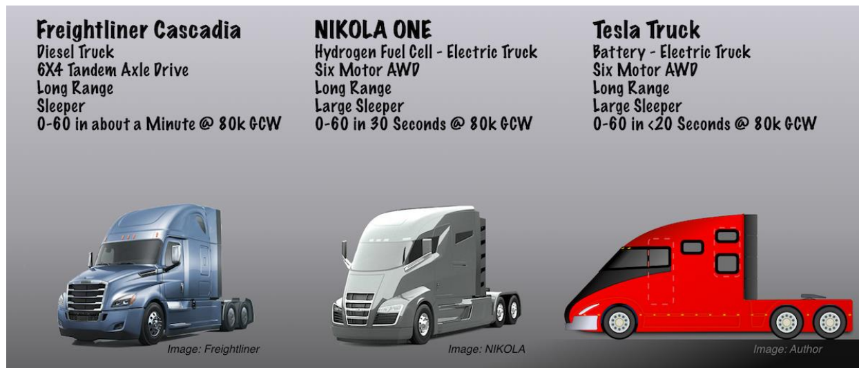
Figure V-18 – Emerging Cleaner Semi-Truck Technologies
