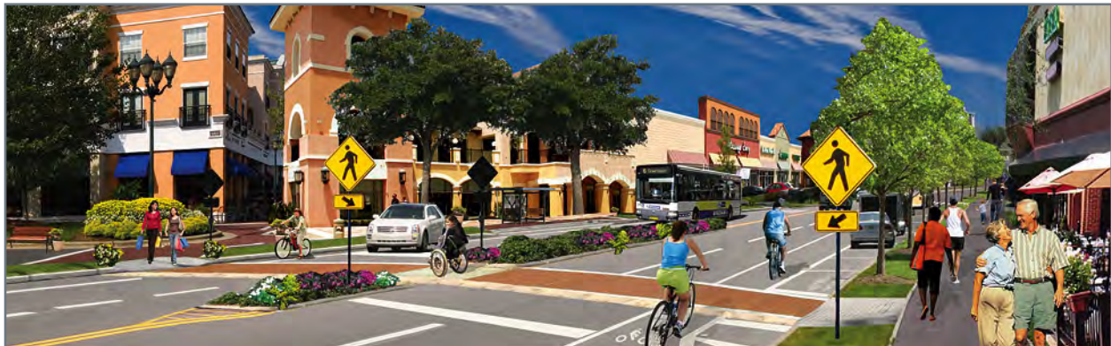
Figure 5.29 Example of intersection with raised pedestrian crossings, pedestrian refuge islands and pedestrian signage.
