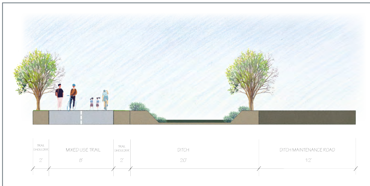
Figure 5.13 Creek Path Cross Section
