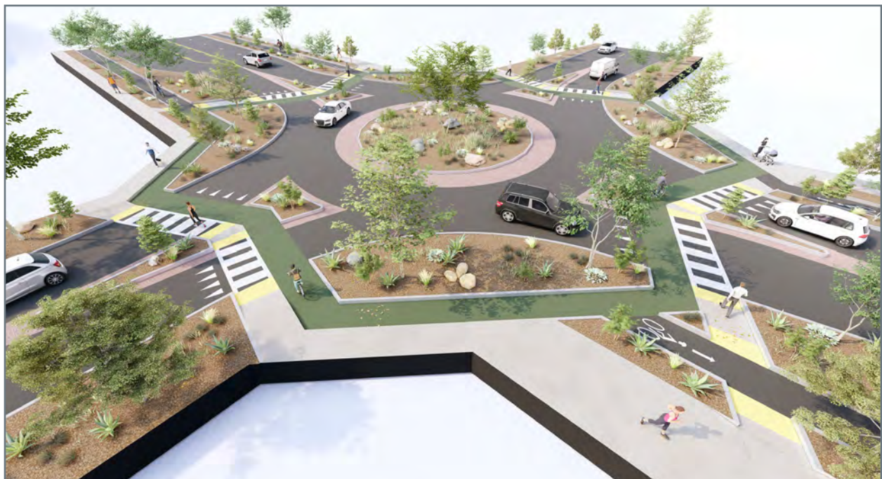
Figure5.1 Proposed roundabout concept for Farmersville & Ash Street/Costner Street Intersections.
