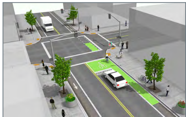
Figure 5.27 Signalized intersection with bike box.
