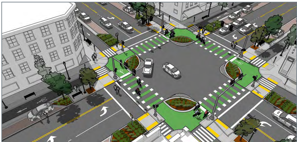
Figure 5.25 Signalized intersection with complete streets concepts incorporated.
